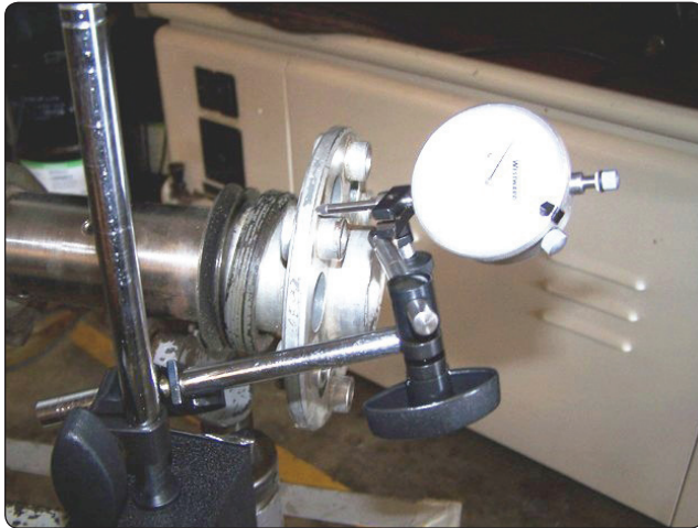
Figure 10-10. Checking crankshaft runout.
