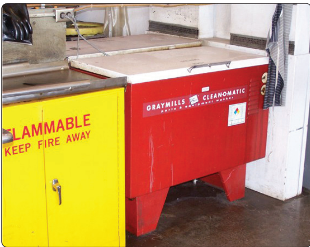
Figure 10-3. Typical solvent degreasing tank.
