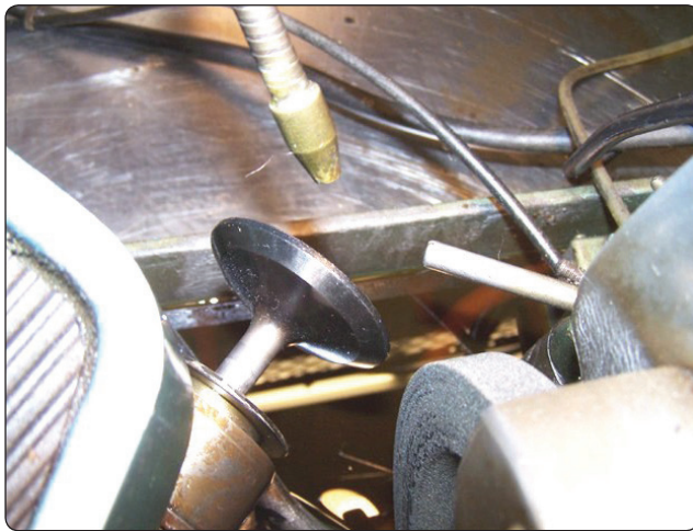
Figure 10-25. Valve in chuck ready to grind.
