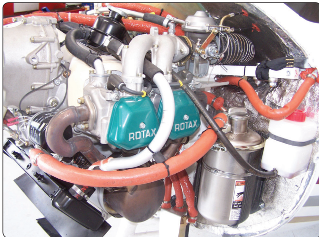
Figure 11-6. Typical four cylinder, four-stroke horizontally opposed engine.
