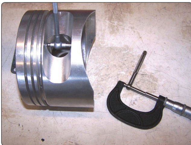
Figure 10-12. Telescoping gauges and micrometer combination.
