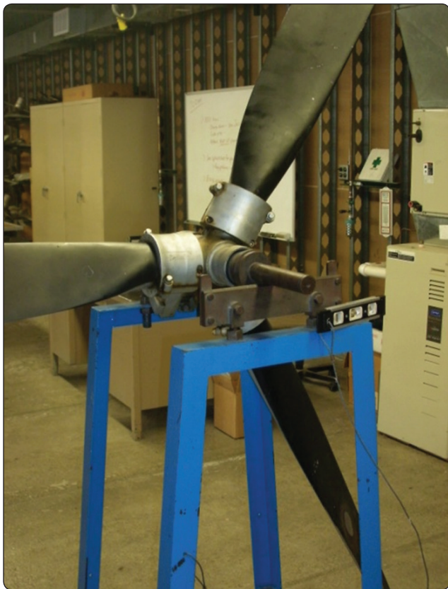
Figure 7-40. Static propeller balancing.
