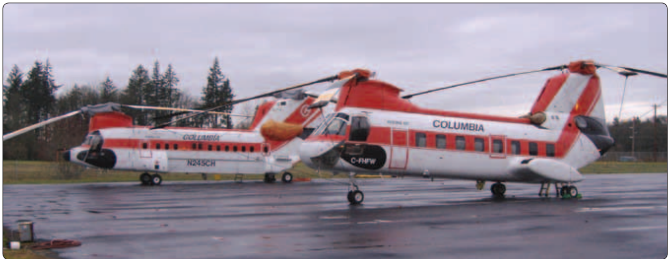
Figure 5-13. Tandem rotor, or dual rotor, helicopters have two large horizontal rotor assemblies, a twin rotor system instead of one main assembly, and a small tail rotor.
