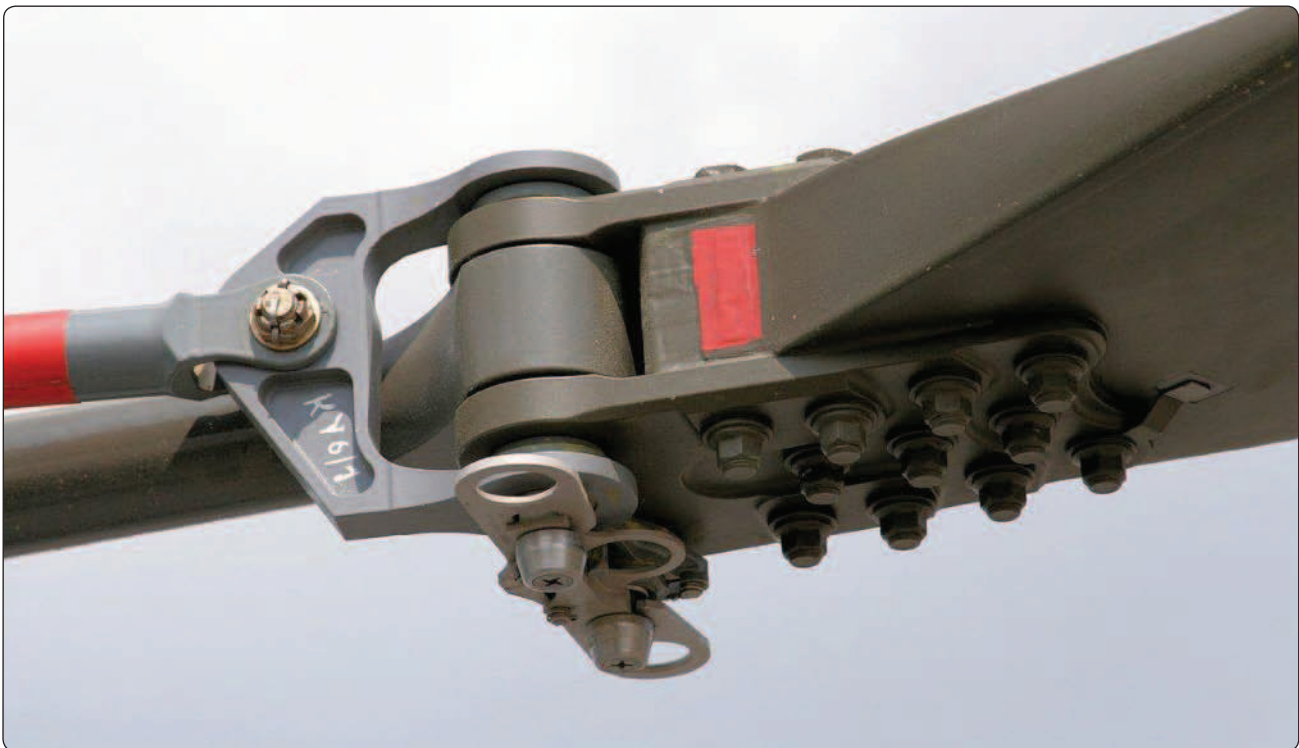
Figure 5-4. Main rotor blade attachment joint on rigid main rotor system.
