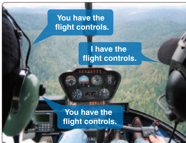
Figure 1-8. There should never be any doubt about who is flying the helicopter.
