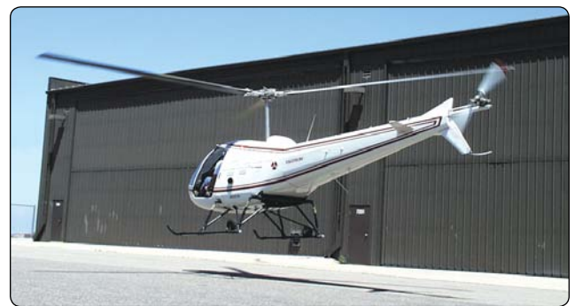
Figure 8-2. Exercise extreme caution when hovering near buildings or other aircraft.
