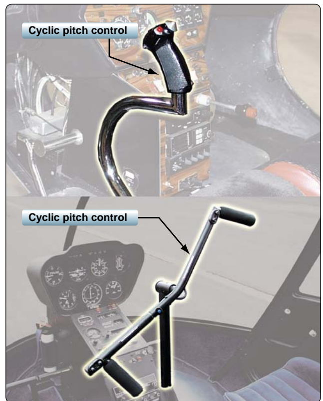
Figure 3-4. The cyclic pitch control may be mounted vertically between the pilot’s knees or on a teetering bar from a single cyclic located in the center of the helicopter. The cyclic can pivot in all directions.
