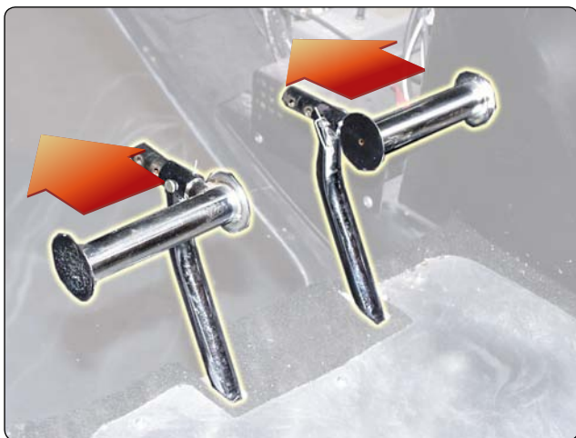
Figure 3-5. Antitorque pedals compensate for changes in torque and control heading in a hover.
