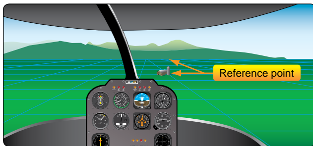
Figure 9-7. To maintain a straight ground track, use two reference points in line and at some distance in front of the helicopter.
