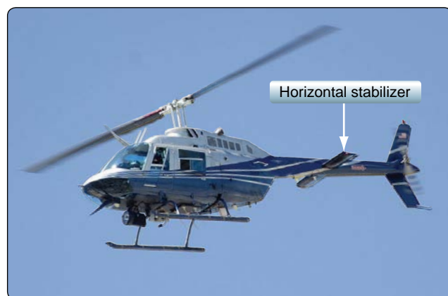
Figure 1-12. The horizontal stabilizer helps level the helicopter to minimize drag during flight.
