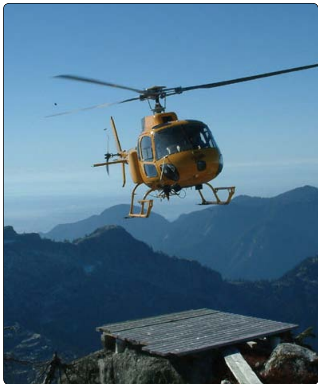
Figure 1-1. Search and rescue helicopter conducting a pinnacle approach.
