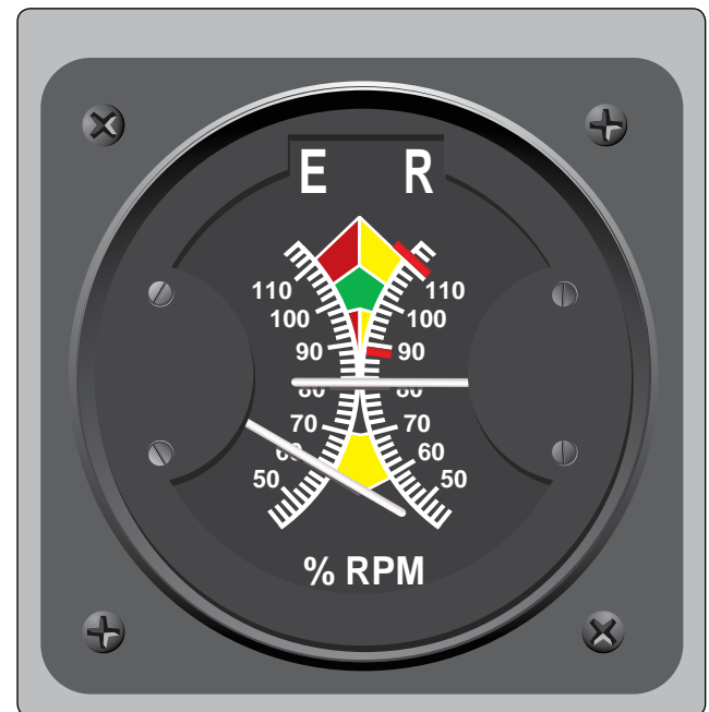
Figure 4-19. A "split" or divided needle condition is a result of a sudden loss of engine power.
