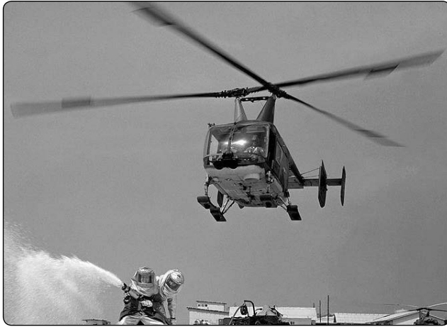
Figure 1-8. HH-43 Huskie with intermeshing rotors.
